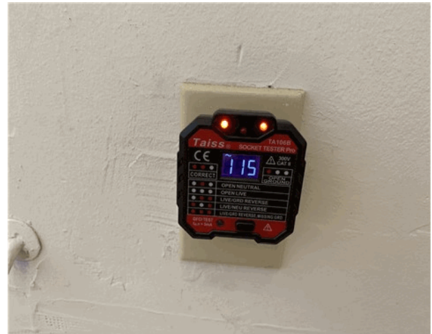
Reverse polarity detected at outlet in back bedroom.
