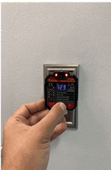
GFCI outlet did not trip in 1st floor.
