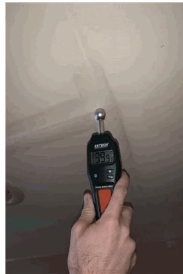
Active moisture detected when tested with moisture meter.
