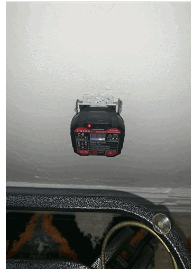
Three prong outlet did not test for grounding in living room.
