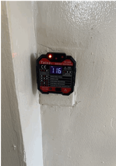
Three prong outlet did not test for grounding in back bedroom.
